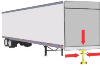
1. Position Auto-Riser under nose of trailer centered from both sides, ensuring the stand is positioned approximately in the middle and a few centimeters back from the nose.
