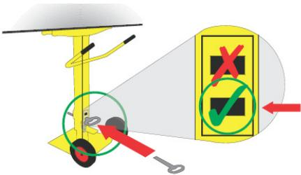
4. Once the Auto-Riser has reached the underside of the trailer, find the appropriate slot and insert the locking pin, locking the unit into place.
