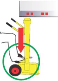
2. Step on the foot plate and press down firmly. You will release pressure on the locking pin. This will allow you to release the locking pin mechanism.
