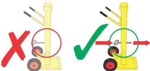
6. Ensure the Auto-Riser is in the correct locked position to avoid potential injury to personnel or damage to equipment. The locking pin should be fully inserted through the centre mast of the stand. If the pin is not fully inserted, repeat steps 3-5.
