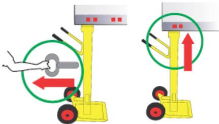
3. To release the locking pin mechanism; pull back on the hand held pin while pressing down slightly on the foot plate. This will allow the Auto-Riser to rise to the underside of the trailer.
