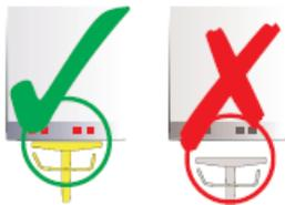
5. Ensure the Auto-Riser is as close to the underside of the trailer as possible (if not making contact). In some cases there will be a small gap between the top of the stand and the underside of the trailer.
